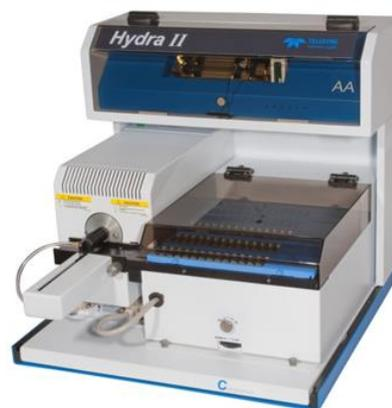
The enhanced moisture control system was used to lower the Method Detection Limit (MDL) by increasing the aqueous sample volume used to determine mercury concentration. To fully investigate the performance of the modified system and the accuracy of the analytical results, the following studies were conducted:
