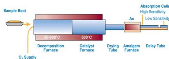
Figure 1. Schematic of Hydra C's Principle of Operation
