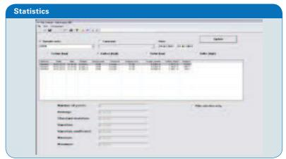
The Statistics screen shows the evaluation of all analyses: Values for average, standard deviation, variance, variance coefficient, minimum and maximum values will automatically be displayed on the screen. An attached printer allows the easy printout of all data and statistics.
