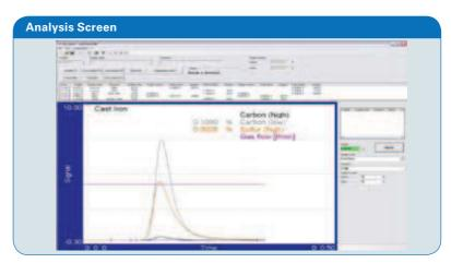
All analysis and peak manipulation tasks can be performed on the Analysis screen. Peak profiles of the current analysis are displayed graphically, while previous analyses can also be recalled and displayed on this screen.
