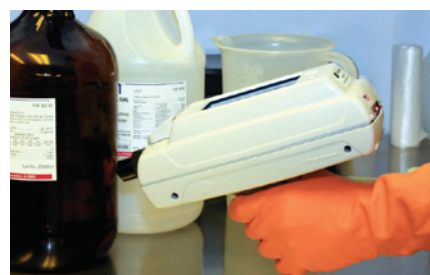
High efficiency optical design allows sampling through amber vials
